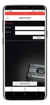
In case your Cellbox 2.0 is equipped with the CBS 21 CFR Part 11 Data Security Software License expand the Login menu by tapping on it and log into the Cellbox 2.0 App with your user login data that have been set on the Cellbox 2.0 device upfront by the administrator user (Admin) that is also used to log onto the Cellbox 2.0 devices using its touch display. This allows you to gather access to your public and your private episodes. To show the episodes press the "READ EPISODES" button.
