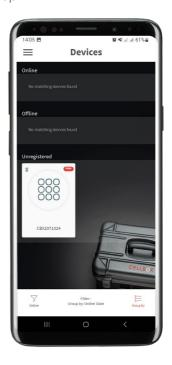
The white tile labelled with the serial number of the Cellbox 2.0 provides you access to start a connection to the respective Cellbox 2.0 device. Tap on this tile and confirm with "OK" to register the device.
