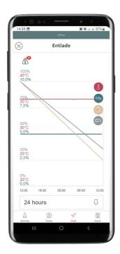
You have the option to change the time range of the graph by pressing the drop down menu on the bottom labelled with the current selected time axis range. The buttons on the upper right labelled with " $\rm CO_2$ ", the temperature symbol and battery meter symbol can be used to show or hide respective curves. You can also scroll sideways to navigate along the time axis.
