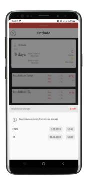
After a while, - the duration depends on the length of the episode, a bar appears showing the progress of data synchronization. Do not remove the mobile device from the vicinity of the Cellbox 2.0 and avoid rotating the display to avoid losing the connection while synchronizing. Also prevent that the mobile device enters any screen saving or display lock mode to ensure that the data set is complete.
